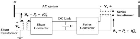
Fig. 1. UPFC installed in a single-machine infinite-bus power system.
