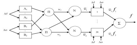
Fig.2 ANFIS architecture for a two-input Sugeno fuzzy model with 20 rules
